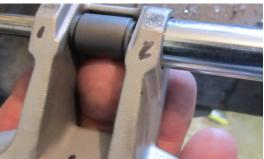
tubular mandrel to allow the pin tool to come back into the tube as the axle is pressed into the roller assembly. Go SLOW and careful!
