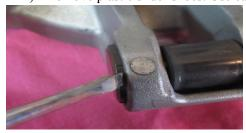
and tiny flat blade screwdriver and use a twisting action. Be careful not to damage the plastic sliders and to keep them in order. It is best to do each arm /roller replacement one at a time....remove the old one, and replace, then move to the next
