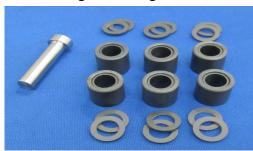
These replacement rollers are built from hardened steel and contain a new custom bushing that has excellent durability and longer life than some of the fibre type bushings in similar applications. These rollers can be used to replace older, worn metal versions, as well as the composite ones in the above applications. When the flyweights in the clutch can shift freely and roll, the result is improved clutch response, backshifting, belt life, and lasting performance.
