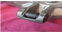
11) Install the spider/governor assembly back into the moveable sheave. **Do not damage the plastic slider shoes.**
