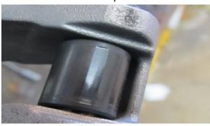
3) Inspect the rollers. It is not uncommon to see flat spots on the plastic rollers, even with limited running. Sometimes all will have it, but sometimes only one or two will have the flat spots.
